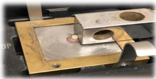
Figure 3: Direct shear strength universal testing machine.
